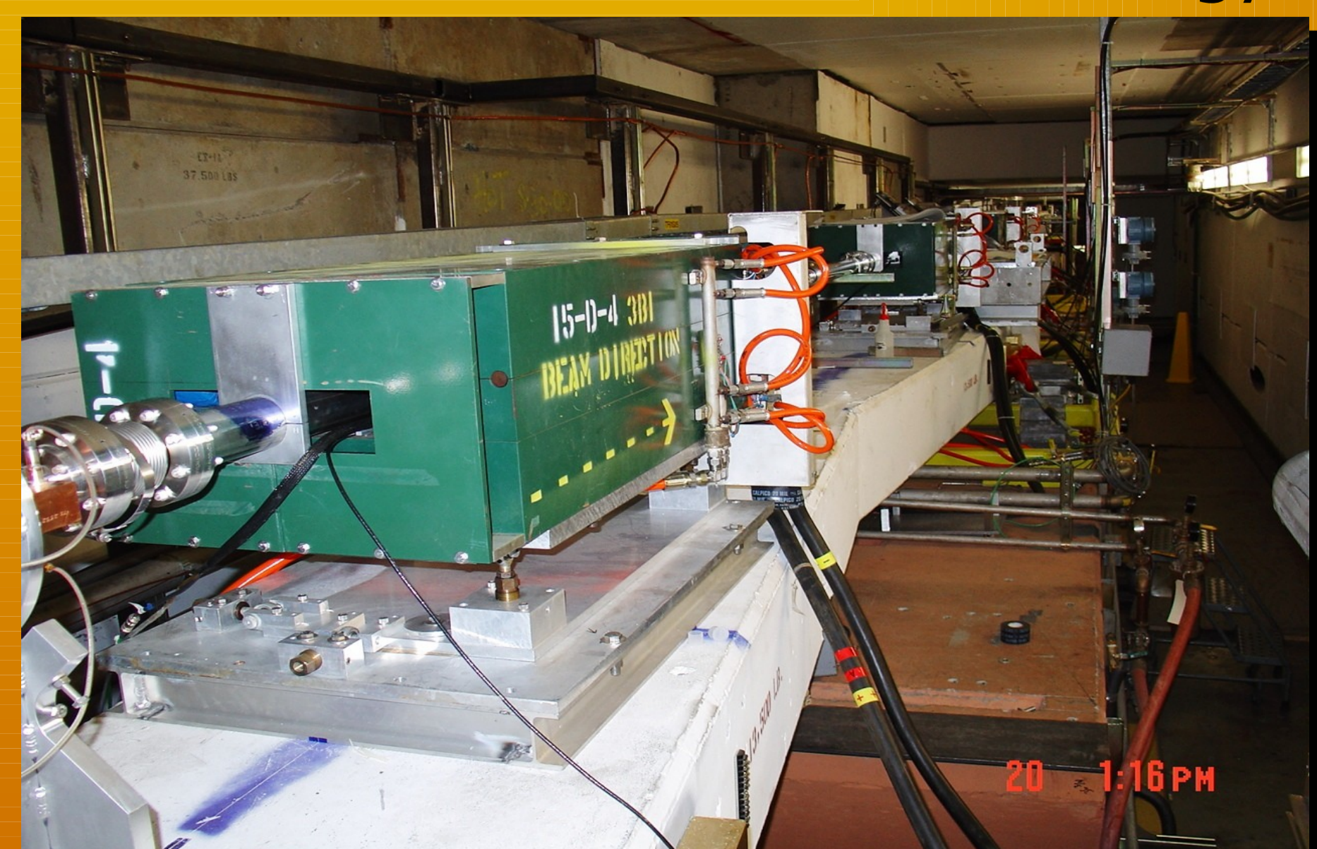
Energy spectrometer BPM prototype, developed at University College London and Royal Holloway University of London
